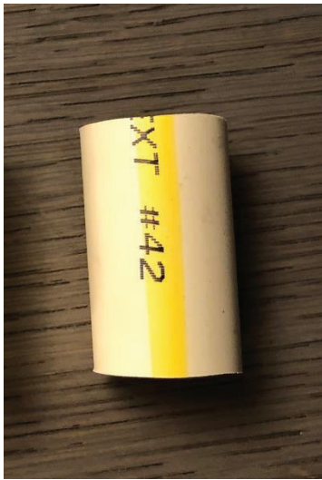
IMAGE 12 - \frac{3}{4} CPVC pipe cut to 4 cm
